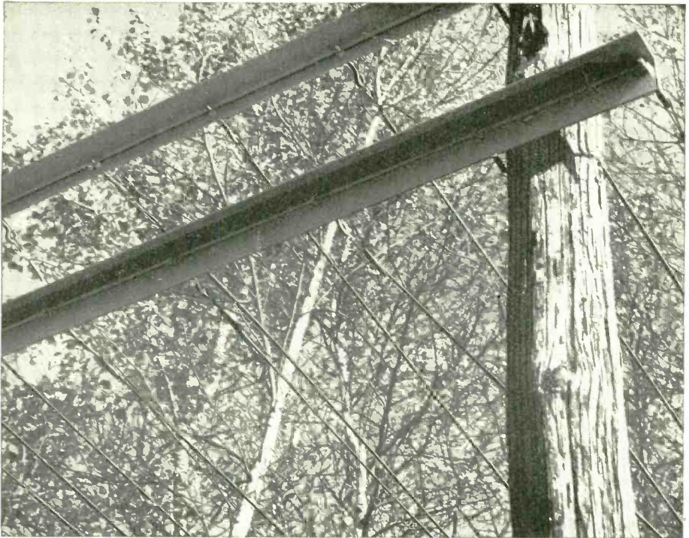
Drop-wire undergoing abrasion tests in birch thicket "laboratory." Below, the new drop-wire, now being installed.
